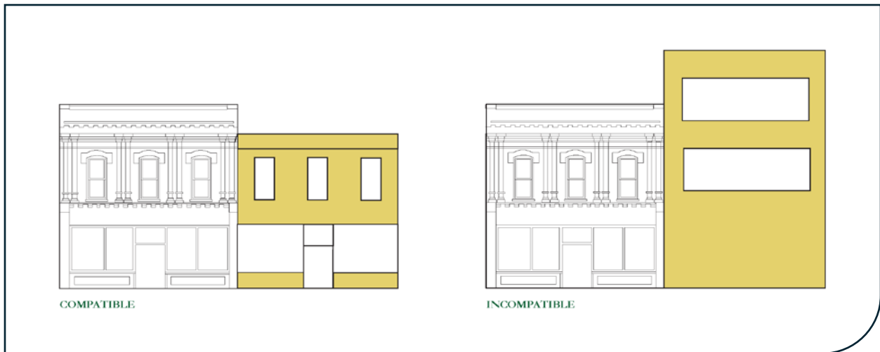
Figure 31: Diagram showing compatible and incompatible new construction style within a block.
