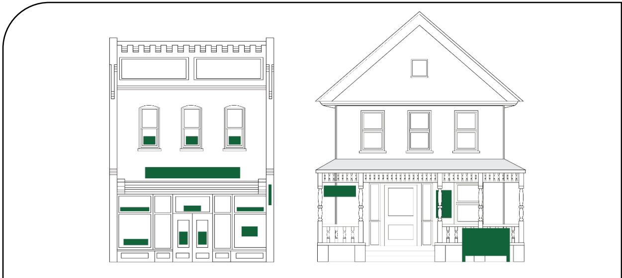
Figure 64: Diagram of possible sign placement on historic commercial buildings and on historic residential buildings adapted for commercial use.
